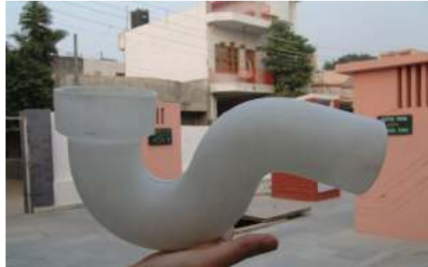
PVC P-trap having 20 mm water seal which does not allow the smell from the pit to enter the toilet
